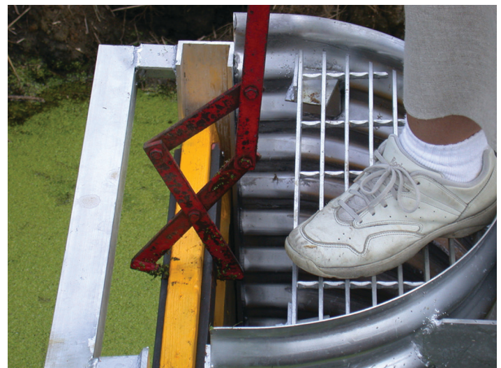
Figure 4. Use of modified ice tongs for removing a board from the structure. Use of a tool such as this facilitates removal/insertion of boards in a safe manner for operators.
