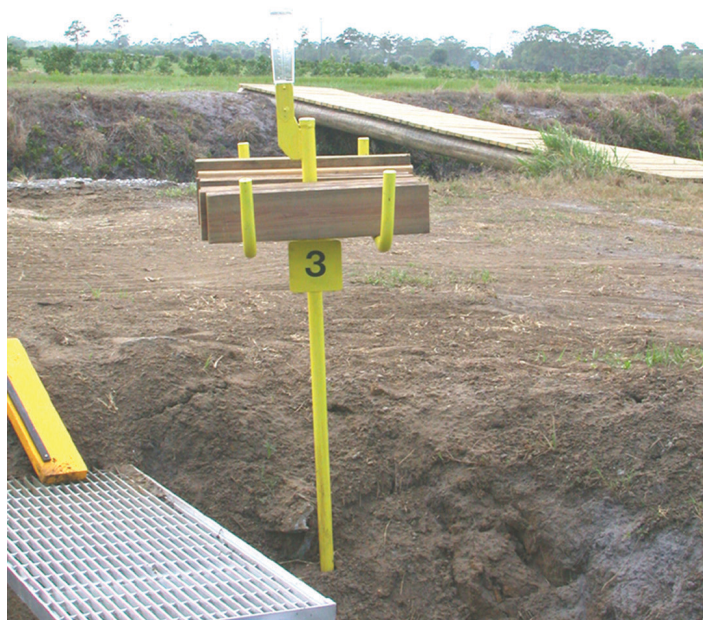
Figure 6. Storage rack for keeping boards readily accessible at the structure. Racks can be numbered for easy reference to structures within the grove. They are also ideal for mounting rain gauges for monitoring rainfall. Credits: PCW
