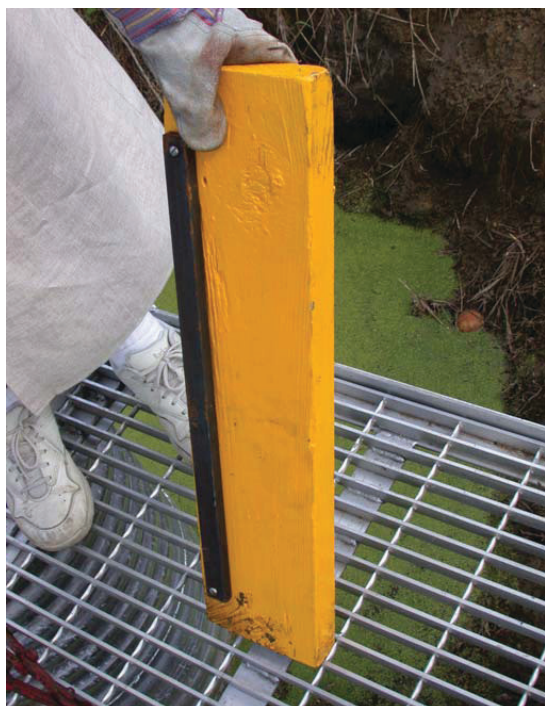
Figure 5b. Wooden sinker board with metal straps attached. Credits: PCW
