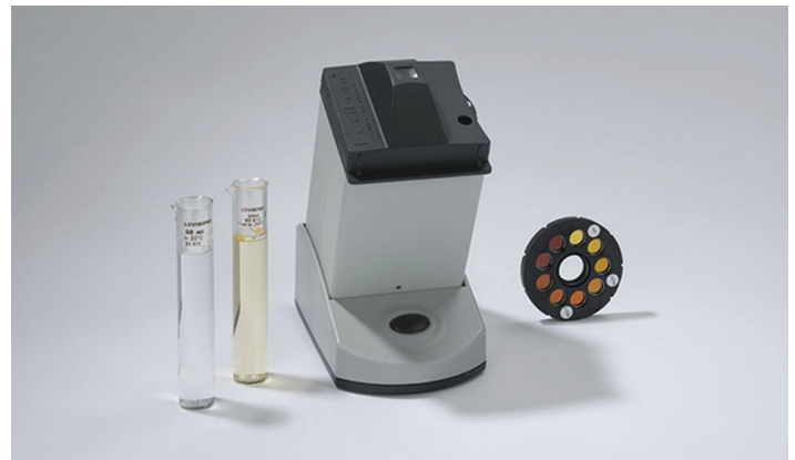
Figure 5. Apparatus used for measuring water color. The tube on the left is filled with distilled water while the tube on the right is filled with the sample. A color wheel is located at the top of the tube on the left-hand side. This wheel is turned until the color of both tubes match. Credits: Orbeco-Hellige, Inc. ( http://www.orbeco-hellige.com )
