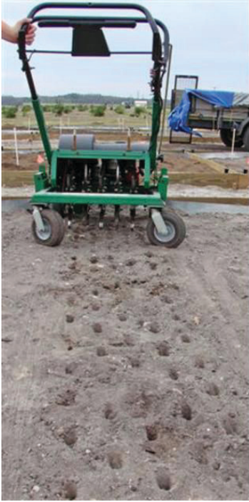
Figure 4. Plug aeration can be used to improve drainage in compacted soils with minimal effect on established plant roots or turfgrass.
