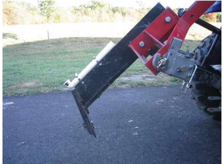
Figure 2. Deep tillage, or subsoiling, requires heavy equipment that can rip soils at depths of 24 inches or more below the soil surface. Credits: Wikimedia Commons
