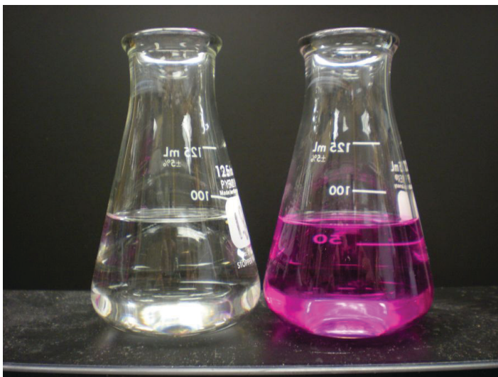
Figure 2. Example of color change exhibited by phenolphthalein indicator dye.
