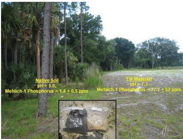
Figure 6. Comparison between native soil and fill material pH and Mehlich-1 extractable phosphorus. The insert image shows samples collected from the upper six inches of the two areas to illustrate the dramatic difference in organic matter content.
