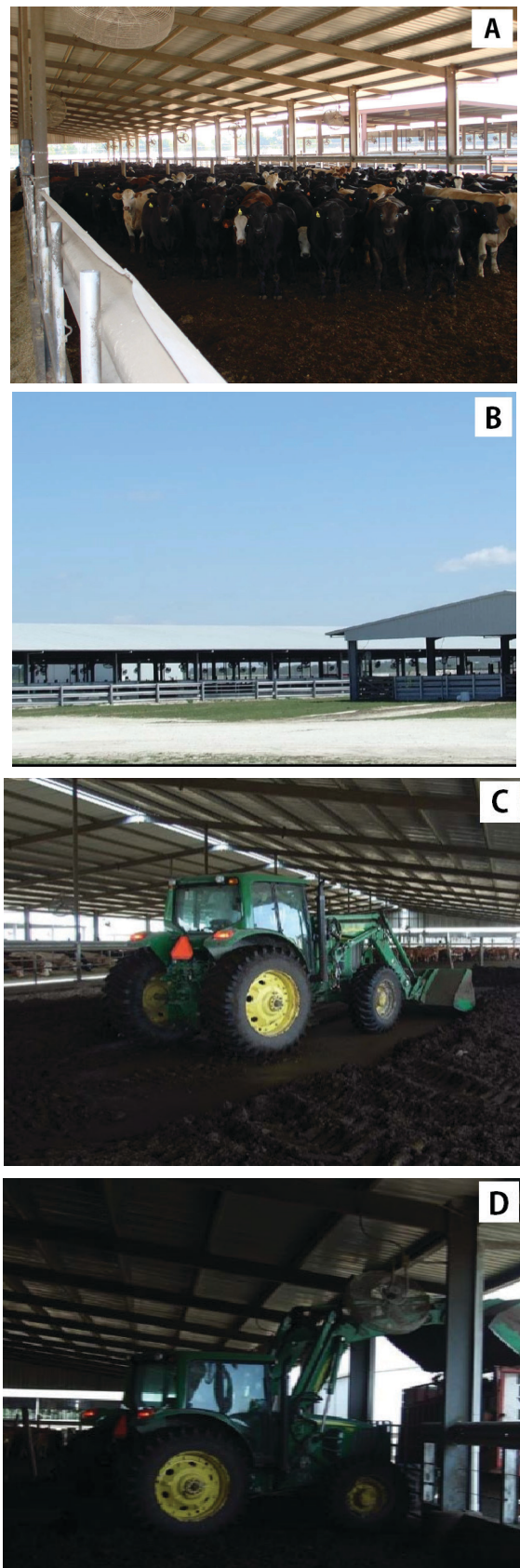
Figure 7. Manure collection: (A and B) Beef feedlot; (C and D) A tractor scraper cleaning the manure and bedding material from the feedlots and then loads the materials into a trailer to be transported to the anaerobic digester unit.
