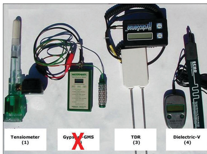
Figure 5. Soil moisture measuring tools currently available for vegetable crops.
