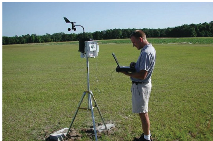
Figure 3. Tools and techniques available to estimate evapotranspiration and irrigation needs: (3.1) weather data may be simply downloaded from a small automated weather station to calculate reference evapotranspiration ( \text{ET}_0 ) and (3.2) water loss in the reservoir of the atmometer mimics \text{ET}_0 .
