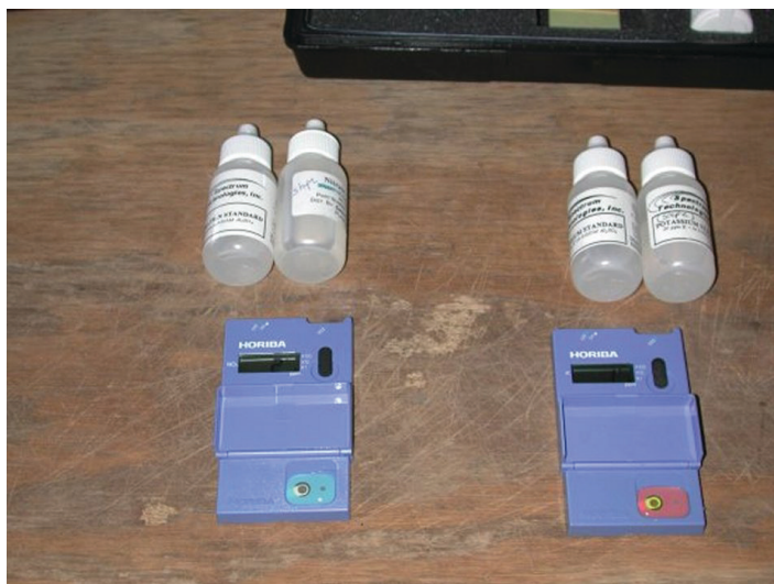
Figure 2. Sap testing for vegetables involves separating the petiole from the leaf blade, (2.1) calibrating the nitrate ( \text{NO}_3\text{-N} ) and potassium (K) ion specific electrodes (Cardi meter shown here) with standard solutions, (2.2) extracting the sap, (2.3) collecting the sap from the press, and (2.4) placing a droplet of sap on the electrode. A hydraulic press may be needed only when few petioles are available or when petioles contain little sap as may occur with strawberry. In most cases, a garlic press will be an adequate tool to extract the sap. Readings should be compared to published sufficiency ranges.
