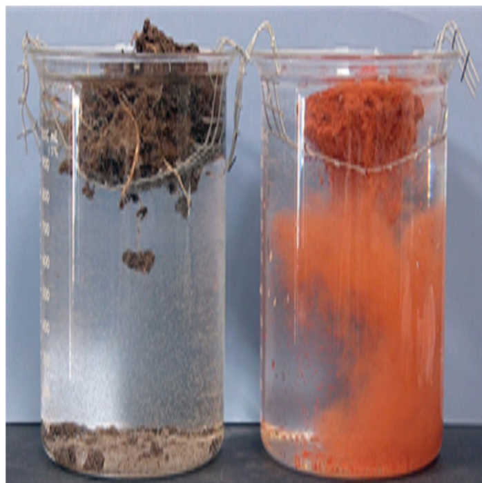
Figure 3. Testing soil aggregate stability.
