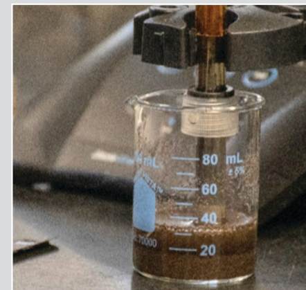
Use testing equipment to gather soil pH readings.
