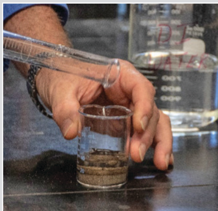
Mix soil and distilled water in a 1:1 ratio by volume.
