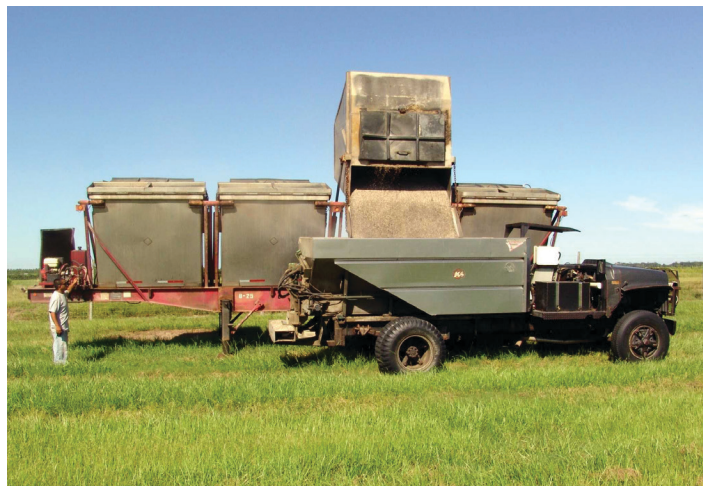
Figure 1. Unloading dry solid fertilizer from a delivery trailer to a grove spreader.
