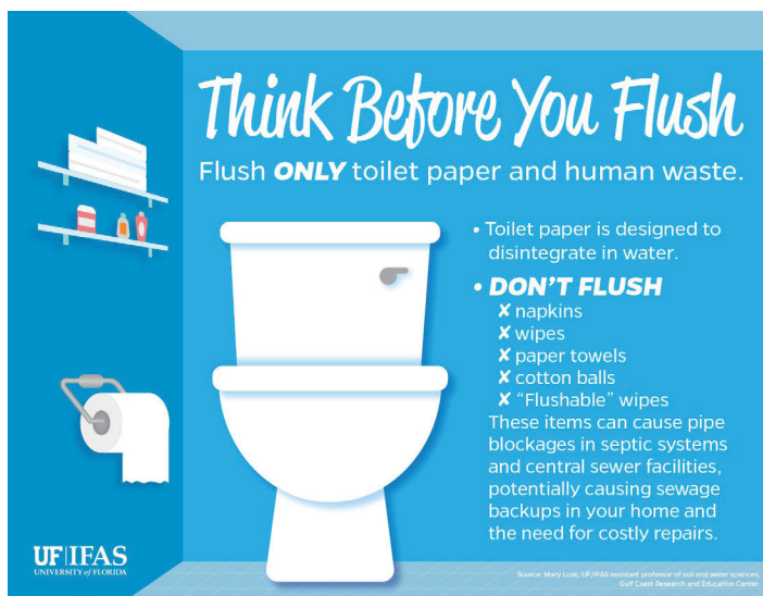
Figure 2. Wipes, including “flushable wipes,” can clog septic systems and public sewers and cause sewage backups in your home.
