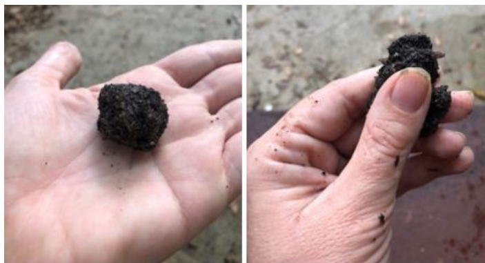
Figure 10. Example of sediment texture analysis. On the left, the sediment has formed a ball. The photo on the right demonstrates the process of forming a ribbon. The ribbon extends less than 2.5 cm from the fingers before it breaks and falls over.
