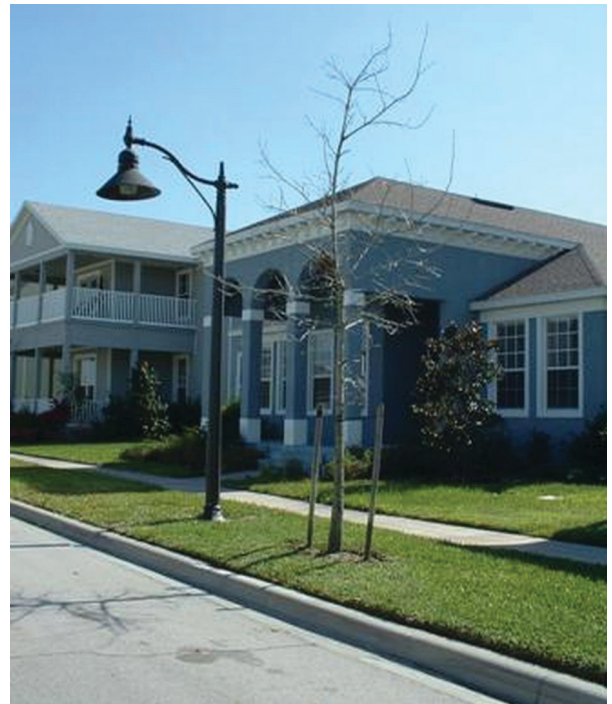
Figure 1. Full cutoff street lights installed along transportation routes in Harmony, FL.
