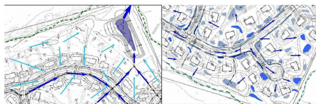
Figure 1. Centralized (left) stormwater management scheme vs. decentralized (right) "LID" scheme. Prince George's County, n.d.
