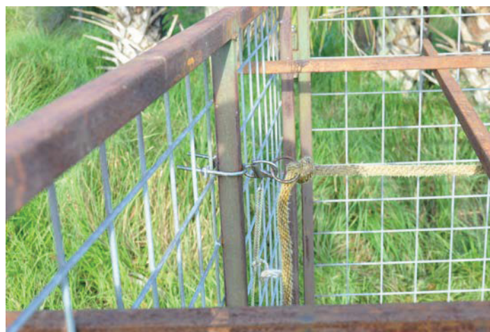
Figure 14. Shackle used with trip wire design in a cage trap. Credits: UF/IFAS, Design by USDA Wildlife Service
