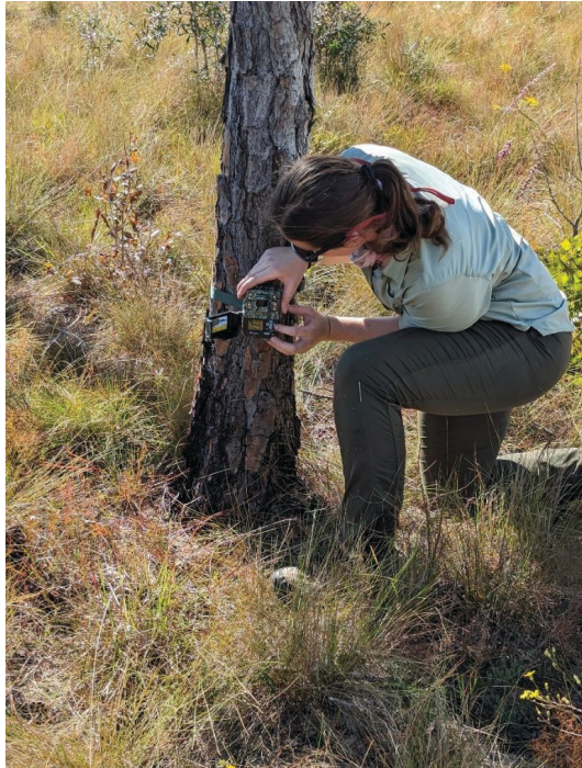
Figure 3. An example of a camera trap being set for the standard setup. Note that the camera is on a vertical tree and is set at approximately the height of the technician's knee.
