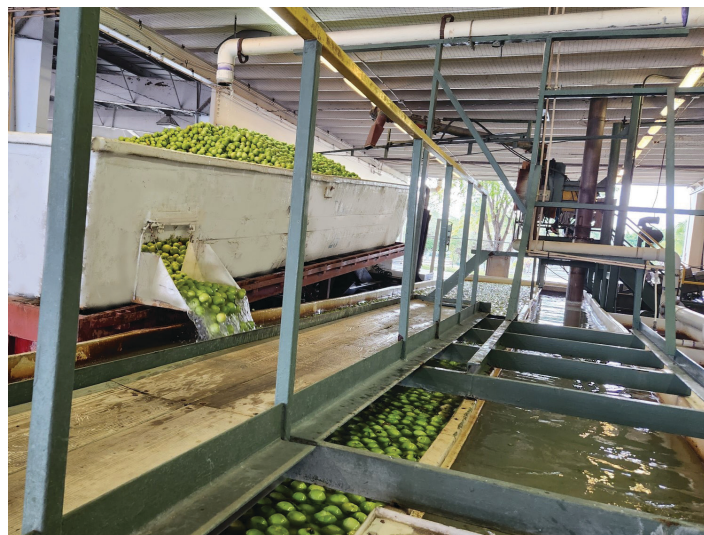
Figure 6. Tomatoes are transferred from gondolas by pumping dump-tank water into the gondola and fluming them out through a side chute into the dump tank.
