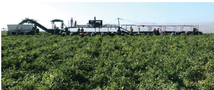
Figure 4. A mobile conveyance system increases hand harvest efficiency.
