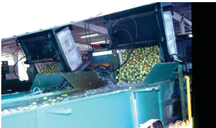
Figure 5. Field bins normally are emptied into a dump tank to minimize mechanical injuries.
