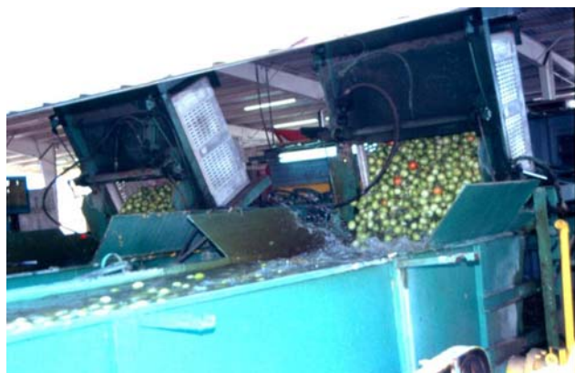
Figure 5. Transfer into a dump tank is commonly used to minimize mechanical injuries. Shown here is transfer from field (pallet) bins into dump tanks. Credits: (J.K. Brecht)
