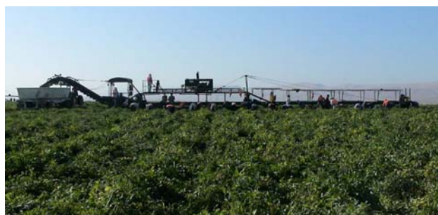
Figure 4. A mobile conveyance system makes hand harvest more efficient. Credits: (S.A. Sargent)
