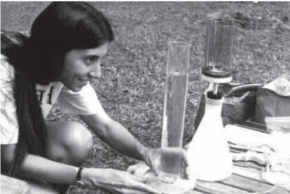
Florida LAKEWATCH volunteer Susan Wright carefully measures water volume in a graduated cylinder before pouring it into the filtration system to the right of the cylinder. This water volume measurement must be accurately measured and recorded.
