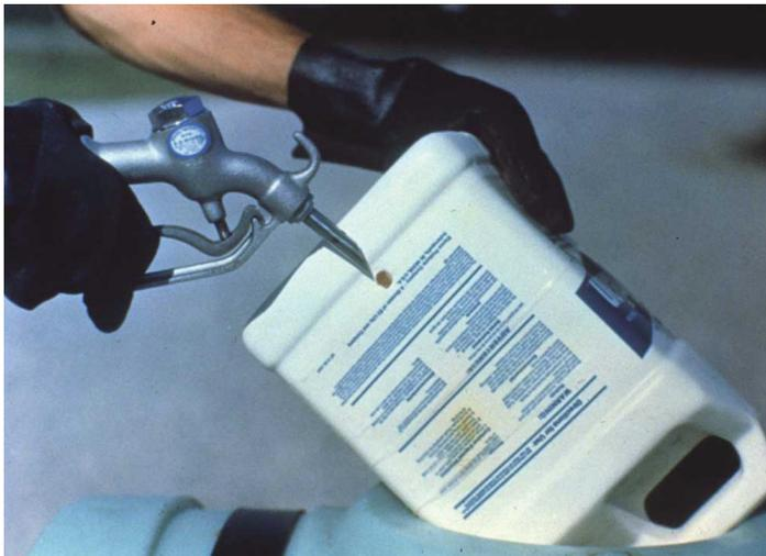
Figure 1. Pressure-rinsing a pesticide container.
