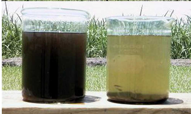
Figure 1. Some effects of high P levels on drainage waters A) proliferation of aquatic vegetation and B) increase in the amount of suspended solids and turbidity.
