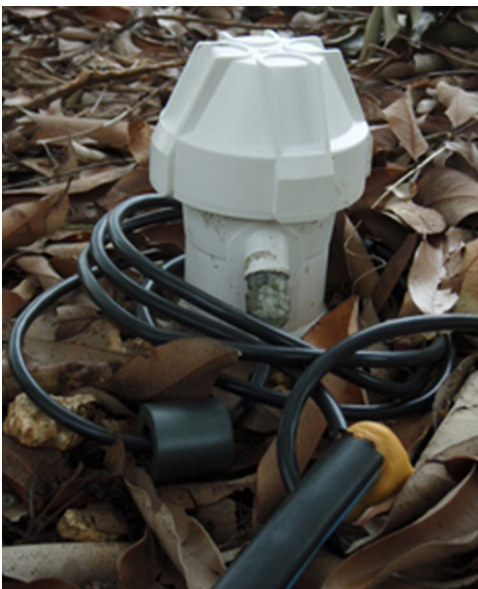
Figure 5. Multi-sensor capacitance probe installed in a south Florida grove. Credits: Luis Barquin
