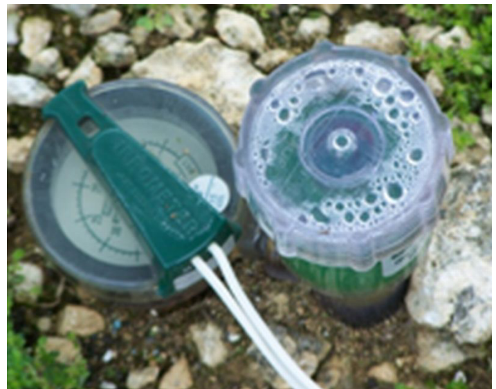
Figure 3. Tensiometer installed in very gravelly loam soil. Credits: Kati Migliaccio
