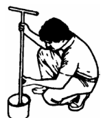
Figure 3. Place 10–15 soil cores into a plastic bucket; mix, dry, and transfer to a bag.
