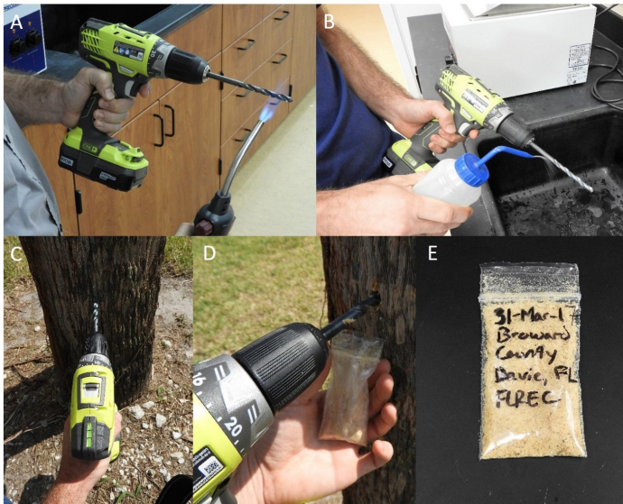
Figure 1. Protocol for palm trunk sampling to test for LY and TPPD phytoplasmas: Heat sterilization of drill bit before drilling for trunk tissue (A), Rinsing drill bit to remove excess tissue/cool after heat sterilization (B), Site selection and removal of the pseudobark so that trunk tissue can be accessed (C), Drilling hole and taking sample of living trunk tissue (D), Properly labeled bag with trunk tissue from symptomatic palm (E).
